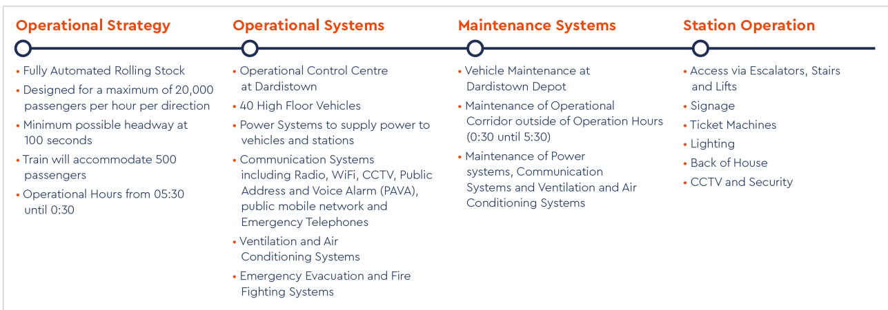
Diagram 17.2: Summary of Key Activities during the Operation Phase of the Proposed Project
